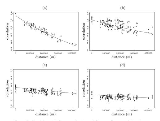
Figure 5. Spatial correlation as a function of distance (in meters) for the Irish wind dataset (open circles: from fitted VAR(3); pluses: empirical) at various temporal lags: (a)  $\tau = 0$ ; (b)  $\tau = 1$ ; (c)  $\tau = 2$ ; (d)  $\tau = 3$ . The solid curve is the stationary correlation function fitted by Gneiting (2002).
